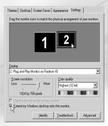
this does not work click the "Advanced" button and look for options like "Horizontal Span" or "Dual View".
